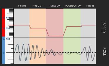
Thanks to specially designed software, POSEIDON proved to reduce up to 60% of the fins drag and consumption, improving the ship speed up to 0.35 knots.
