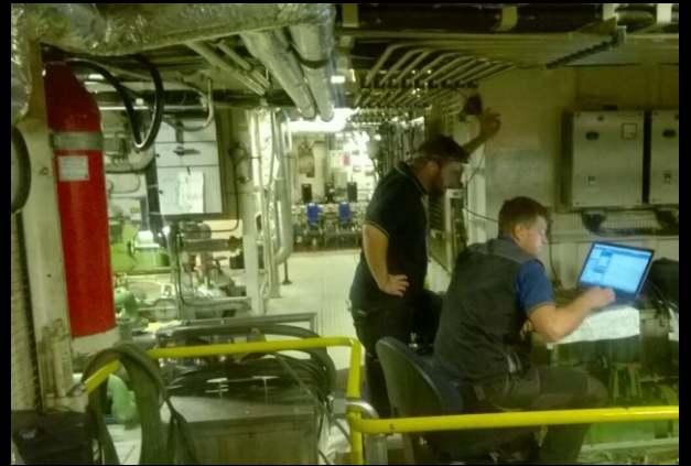
On board Service with specialized service engineers tuning Stabilizers Power Unit
